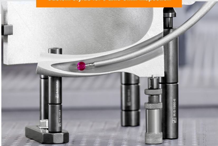
Custom stylus for 5-axis CMM inspection
